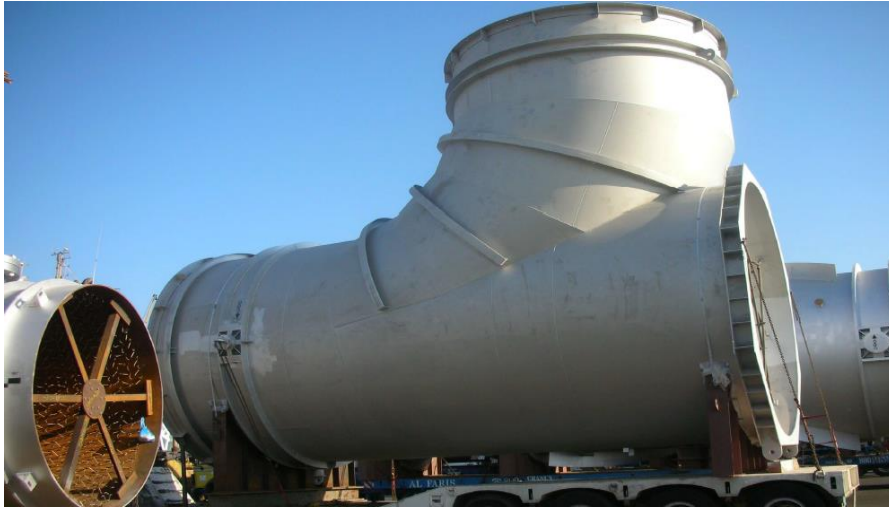
Boiler Stack and Flue Gas Duct for JGC (Saudi Arabia)
